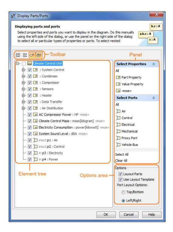
The following procedure will guide in working with the **Display Parts/Ports** dialog when you want to display required ports and properties on the diagram pane.
