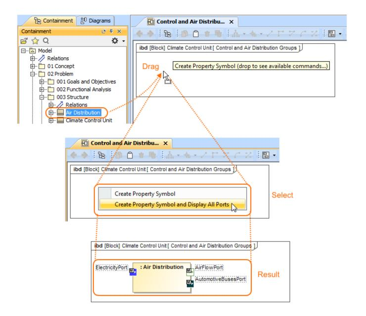
You can display a Part Property shape by dragging a Part Property element from the Model Browser to the SysML Internal Block diagram pane. If this Part Property has ports defined, you can display them by using the long drag, and selecting an appropriate option from the opened menu (see Example 4).
