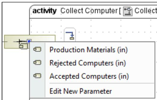
If a parameter with an *inout* direction is selected for the Activity Parameter Node creation, then two Activity Parameter Nodes are created on the diagram frame.
