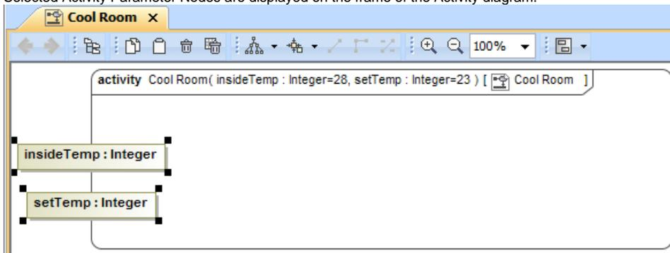
If you want all Activity Parameter Nodes to be displayed automatically when creating a new Activity diagram, go to **Options > Project** on the main menu, and set the **Display All Activity Parameter Nodes in Diagrams** option to *true*.
