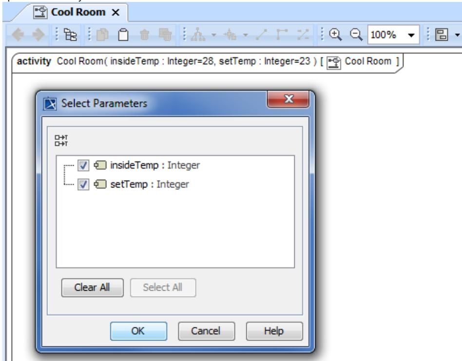
2. In the opened **Select Parameters** dialog, select the parameters that you want to display, and click **OK**. Selected Activity Parameter Nodes are displayed on the frame of the Activity diagram.
