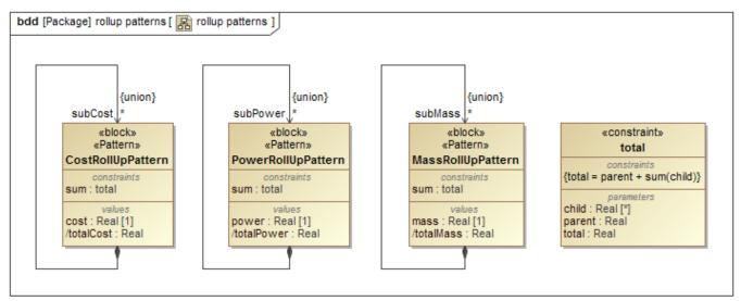
The total cost, mass, or power rollup pattern Blocks defined in the SysML Block Definition Diagram.
