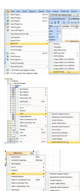
2. You can export either (i) elements of a class mapping by selecting a class mapping from the treeview, see first figure below or (ii) instance specifications of a schema class by selecting a schema class from the treeview, see second figure below.
