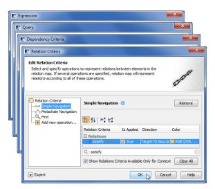
The layout of the dialog is the same in all the described cases. On the left side of the dialog, you can select an operation type that best suits for specifying the needed criterion. Selecting an operation type opens the criteria specification panel on the right side of the dialog.
