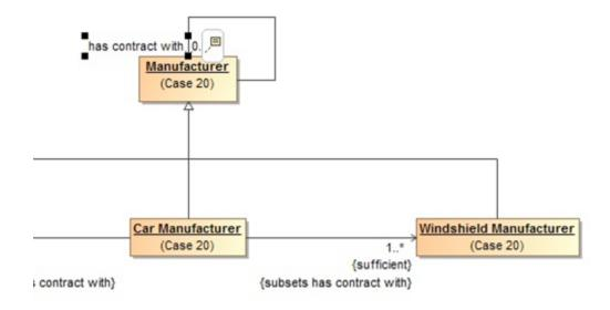
The Concept Modeler highlights the subsetted property on the selected diagram.
