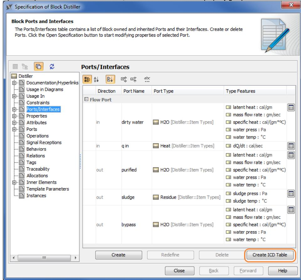
The Blackbox ICD Table is created. All external Ports/interfaces of the selected Block are represented in the table automatically. [Learn more about Blackbox ICD Table >>](#)
