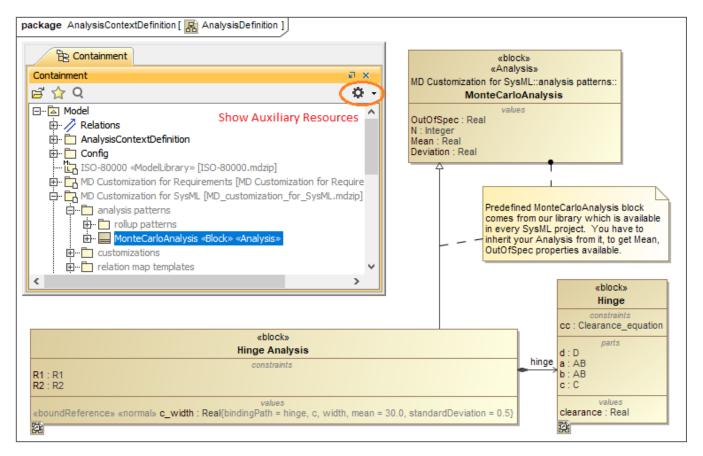
Inheriting the Hinge Analysis Block from the predefined MonteCarloAnalysis Block and setting the Hinge Block as part of the Hinge Analysis Block.
