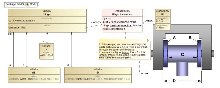
The Block Definition diagram of the Hinge model with distributed value properties applied.
