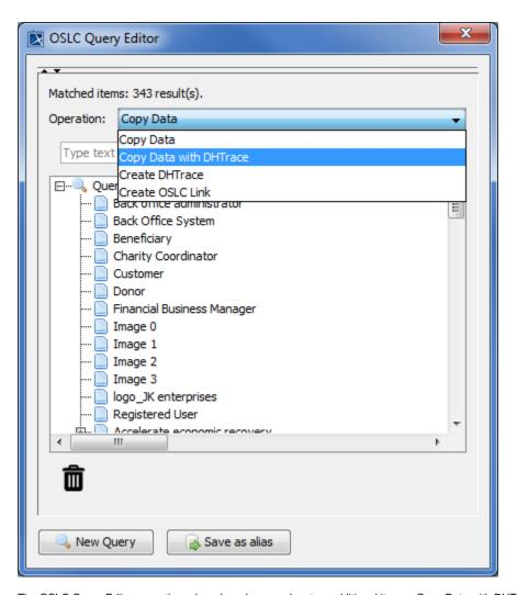
$\label{thm:condition} \textbf{The OSLC Query Editor operations drop down box now has two additional items - Copy Data with DHTrace and Create DHTrace... } \\$
