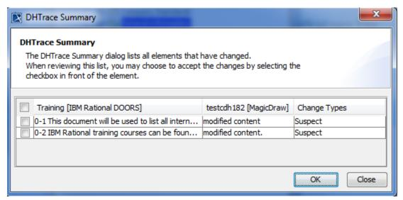
A new dialog has been added called the DHTrace Summary dialog which allows a user to clear Suspect DHTrace links. This dialog can be invoked by performing Check Changes -> Check DHTrace Changes Recursively.
