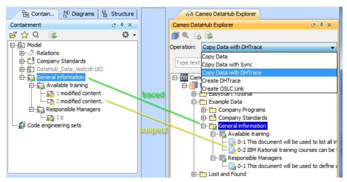
In Trace relations, there is a link relationship between source and target nodes. When either of the nodes undergoes any change, the trace relationship is marked with a Suspect status. This status can be cleared or the DHTrace can even be removed if the traceability feature is no longer needed.
