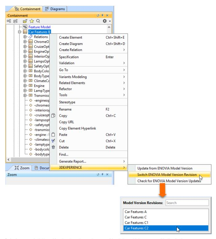
During the process of switching revision, the main goal is to retain as many of the existing model elements as possible, changing them as necessary instead of deleting and re-creating them. Only the Product Configurations (Instance Specifications) will be added anew.
