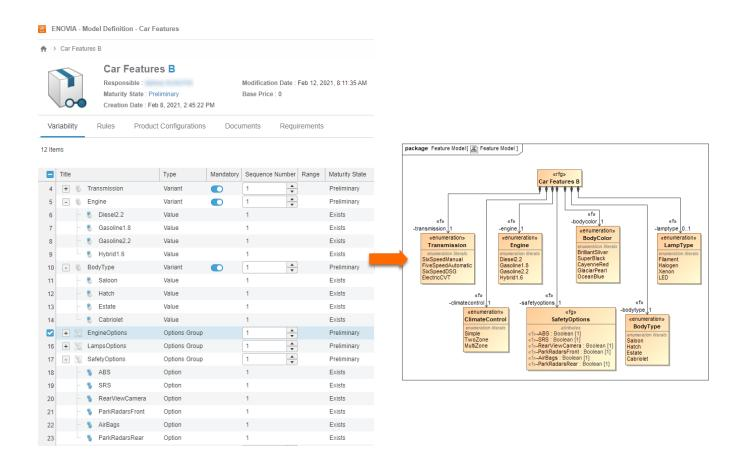
The Product Configurations in the modeling tool project are imported as UML Instance Specifications. You can also display them in the diagrams.
