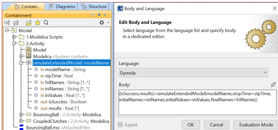
2. Create a Call Behavior Action in an Activity diagram of a Block and create valid in/out Parameters through in/out Pins according to the parameters of the Opaque Behavior. You can also create a Block, e.g., *Modelica*, with value properties to keep values and set an Activity as the Classifier Behavior of the Block as shown below.
