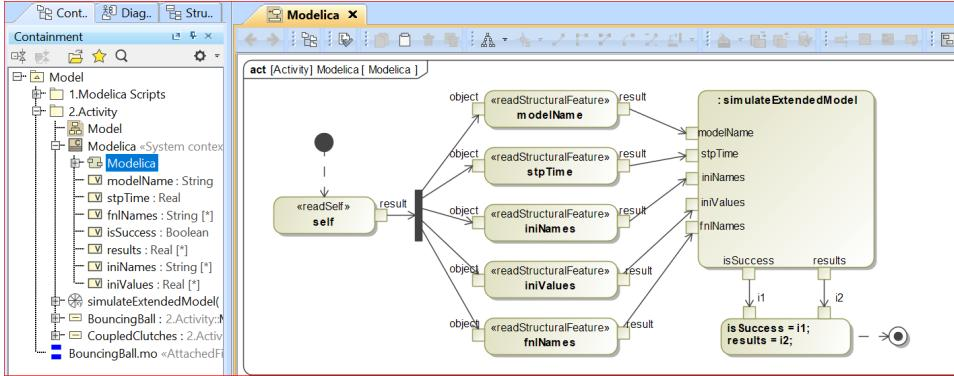
3. Create an Instance Specification to specify parameter values, e.g., *CoupledClutches*. Run the simulation through the instance to get results from Dymola back to Simulation as shown below.
