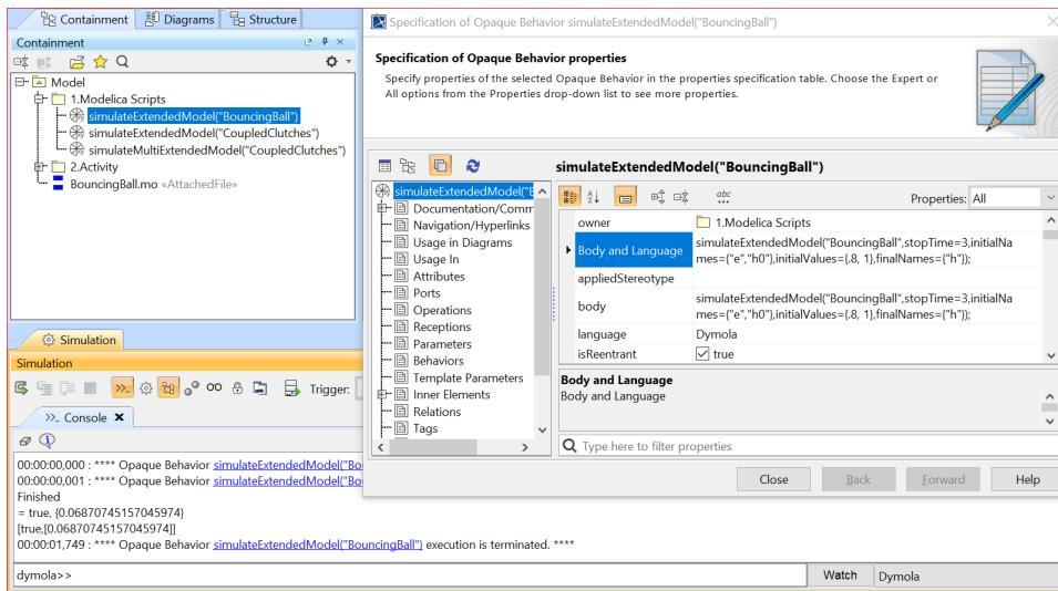
Results from the simulateExtendedModel of Dymola called from an Opaque Behavior.
