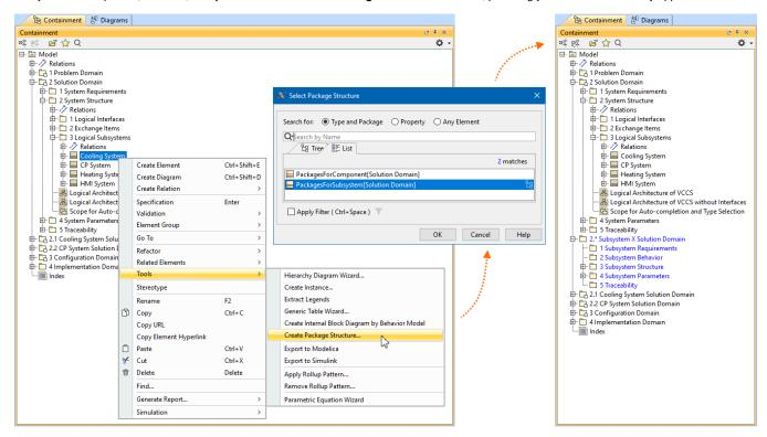
Creating a MagicGrid-based package structure via the Create Package Structure command.
