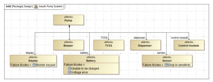
In this Block Definition Diagram, the Display, Battery and Sensor blocks have specific Failure Modes linked to them.
