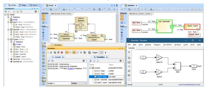
The Simulink co-simulation result from the system which has two Simulink models (GainAdd.slx and Gain5.slx) connected via Flow Ports.
