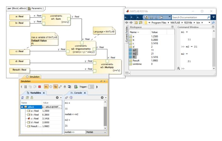
Variables in the shared MATLAB workspace can be used in either Simulation Toolkit or MATLAB.
