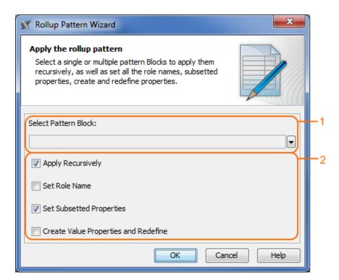
The Rollup Pattern Wizard when trying to apply a rollup pattern for a Block. Two areas of the wizard are highlighted: 1- Select Pattern Block, 2 -Options.
