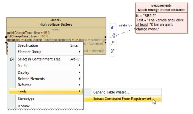
After selecting the **Extract Constraint From Requirement** command, the constraint {distanceOnQuickCharge >=70.0} is automatically created. It satisfies the requirement text "at least 70".
