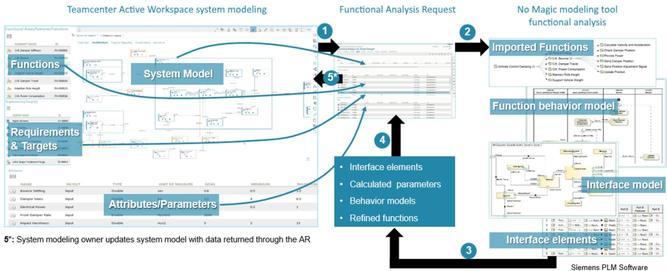
Assembling the Analysis Request to import to the No Magic modeling tool for functional, interface or parametric analysis.
