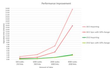
A line chart of performance improvement of DataHub 19.0 compared to the 18.5 version on importing and synchronization with changes.
