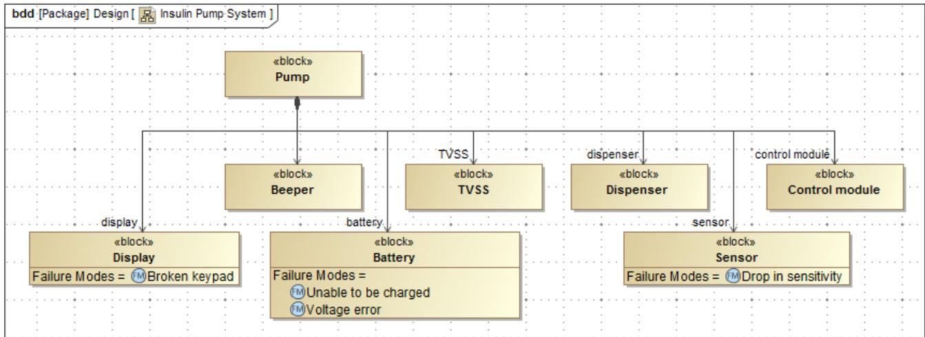
In this Block Definition Diagram, the *Display*, *Battery* and *Sensor* blocks have specific Failure Modes linked to them.
