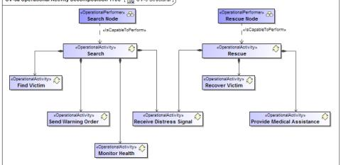
OV-5b diagram for Operational Activity flows. This diagram is based on the UML Activity diagram. nal Activity Model [ 📸 Search & Rescue ] OV-5b Operation
