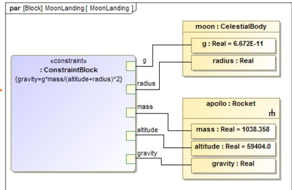
The main steps, highlighted in orange, in the Parametric Equation Wizard when creating the SysML Parametric Diagram from mathematical equation.
