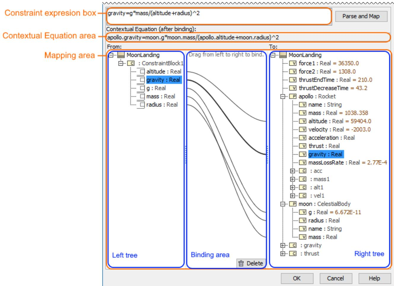
Three main areas (highlighted in orange) in the Parametric Equation Wizard: constraint expression, contextual equation, and mapping. The mapping area contains the left and right trees and binding area.
