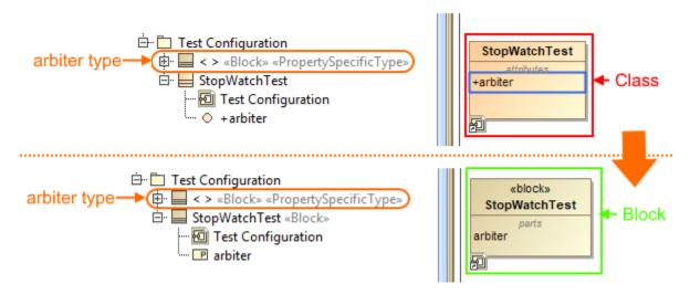
The arbiter property is typed by the PropertySpecificType is owned by the StopWatchTest Block.
