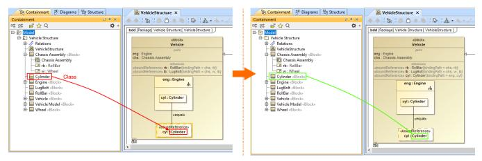
The cyl Reference Property is typed by the Cylinder Block.
