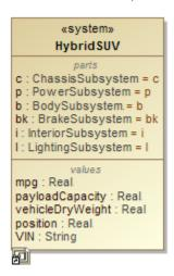
Visibility representation. SysML, properties and operations of the Block are public. Visibility representation literals, like +, #, ~, -, are not displayed in the Containment tree or in the element symbol on a diagram.
