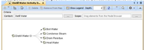
Structure Decomposition Map displays the decomposition of the Part Properties related through the Composition relationship of the specified
