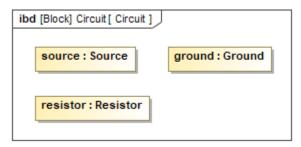
The Circuit IBD consists of three parts: source, ground and resistor.
