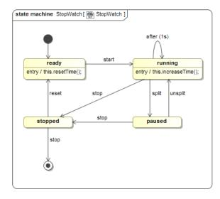
At this point the *StopWatch* has been completely modeled. You can now execute the *StopWatch* Class using Cameo Simulation Toolkit.
