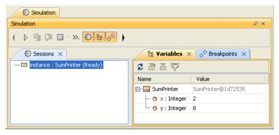
4. The simulation will be suspended when pin **a** or **b** of the **print** action is activated. You can hover your mouse pointer over the active element to see its runtime value.
