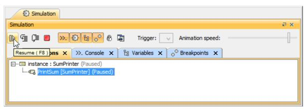
6. The simulation will be suspended again when pin **b** is activated. Click the **Resume** button to continue the simulation. In the **Console** pane of the **S imulation** window, you can see the printed value of 10, which is the summation between 2 and 8.
