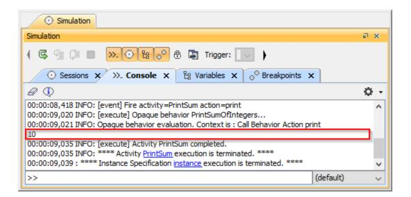
Note to do not want to display animation (silent simulation), you can create **Simulation Configuration** to customize the simulation, select **instance** as the **simulationTarget**, and set **silent** to **true**. See Simulating a Simulation Configuration and Simulation Configuration and Ul modeling for more information.
