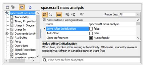
3. Run simulation via the Simulation Config. All related results will not be calculated automatically, so you need to manually invoke it via the Refresh in Variables pane or Start (F8) (see the following figure).
