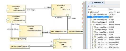
4. Select **true** for the **Solve After Initialization** option, and run the Simulation Config. All related results will be calculated automatically (see the following figure)
