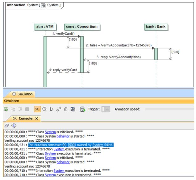
A Sequence diagram showing how a Duration Constraint (500) can be used to evaluate between the Call Message and Reply Message.
