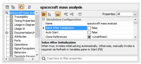
3. Run simulation via the Simulation Config. All related results will not be calculated automatically, so you need to manually invoke it via the Refresh in Variables pane or Start (F8) (see the following figure).
