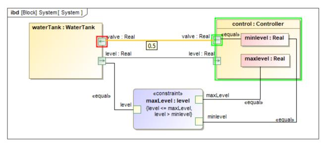
Animation of value propagation in the Internal Block diagram.
