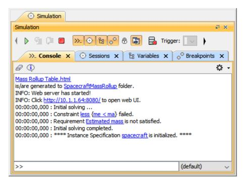
The Console messages appearing in the Simulation Console with the filter Options set to Warn.
