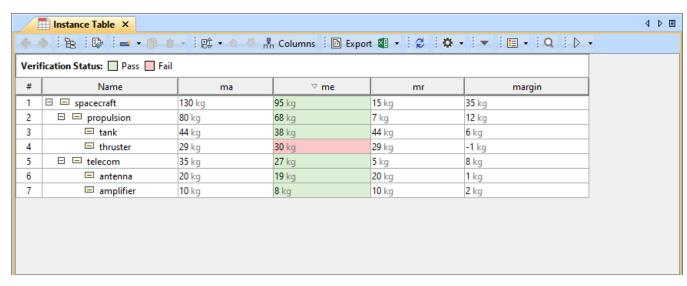
Value verification status is displayed in an Instance Table without using the Simulation Profile.
