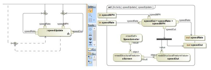
The model uses an activity to encapsulate a fork node
