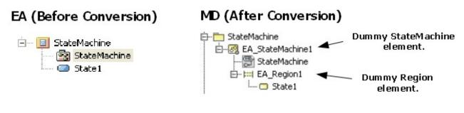
A dummy StateMachine element and a dummy Region element.
