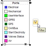
2. In the smart manipulator toolbar, click T. The diagram is filtered by all items specified in the Legend, meaning that all diagram aspects are either hidden or displayed.
