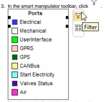
The diagram is filtered by the selected Legend item, meaning that the diagram is limited to one specific aspect. If the filtering preference is *Show*, the diagram displays only the element symbols filtered by the Legend item, while the rest of the element symbols are hidden. If the filtering preference is *Hide*, the diagram hides the element symbols filtered by the Legend item while the rest of the element symbols are displayed.
