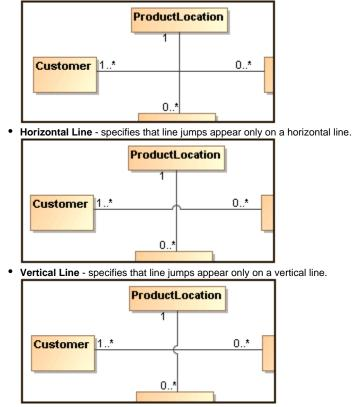
(i) The line jump changes are applied for the current diagram only. To change line jumps for the whole project, see Formatting symbols.
