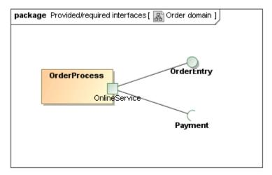
In the Composite Structure diagram, you cannot draw provided and required interfaces themselves, but, with the new functionality of MagicDraw, you can display a preexisting port with the required and provided interfaces as images.
