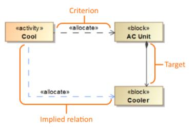
In the example above, the value of the **Target** parameter is a generalization (direction – **Target To Source**). This means that starting from the *AC Unit* block, all composed blocks are collected. In this case, the *Cooler* block is the result of the **Target** parameter. By default, the values of the **Tar get** parameter are simple navigation operations - a generalization (direction - **Target To Source**) and part (direction - **Target To Source**).
