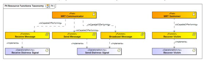
· P4 Resource Functions diagram for Function flows. This diagram is based on the UML Activity diagram.
