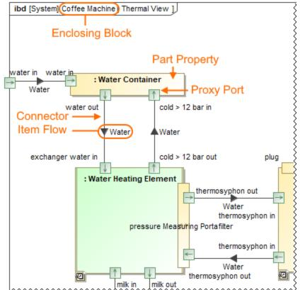
An internal structure of Coffee Machine Block where Part Properties are connected via Proxy Ports by using the Connector.
