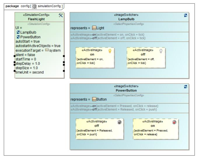
Using ImageSwitcher in the FlashingLight.mdzip sample with internal simulation clock.
