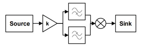
This example portrays the signal flows between system components. The signal flow is unidirectional, and physical conservation laws do not apply in these applications because the same signal can be sent to multiple receiving components. In this model, the function generator is being amplified and then sent to parallel filters (one high-pass filter and one low-pass filter), until the mixer combines the filtered signals for the final
