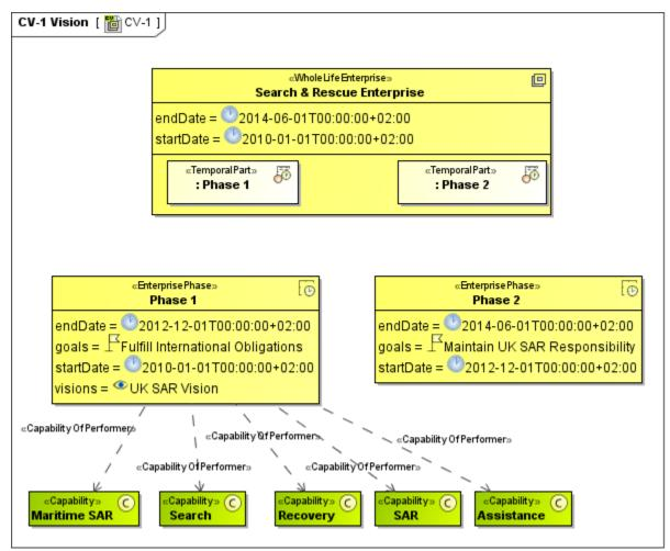
CV-1 provides a high-level scope for the Architectural Description which is more general than the scenario-based scope defined in an OV-1.
