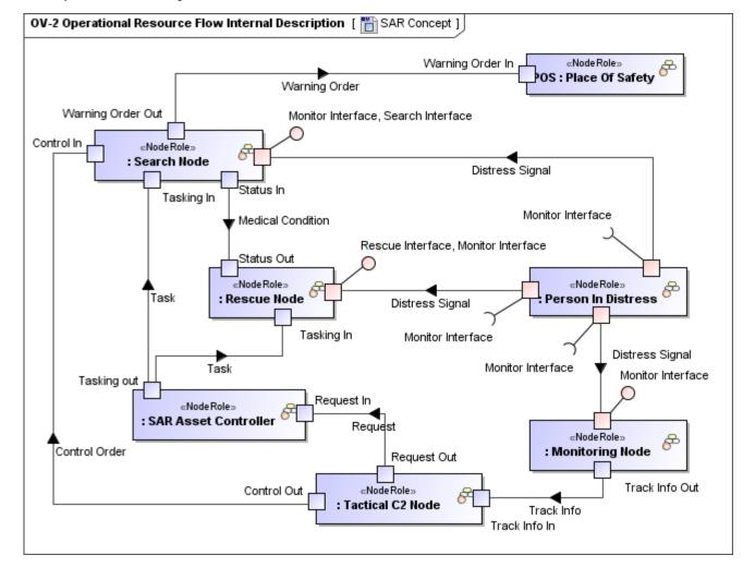
The Needlines established in an OV-2 can be realized by resources and their interactions in a SV-1 Systems Interface Description model or SvcV-1 Services Context Description model.
