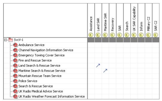
This model is analogous to the SV-5a Operational Activity to System Function Traceability Matrix – but provides the interface between Capability and Service Models rather than Operational to System Models.
