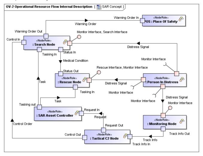
The Needlines established in an OV-2 can be realized by resources and their interactions in a SV-1 Systems Interface Description model or SvcV-1 Services Context Description model.
