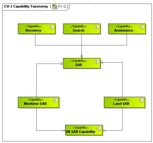
The CV-2 is used to capture and organize the capability functions - required for the vision set out in the CV-1 Vision.
